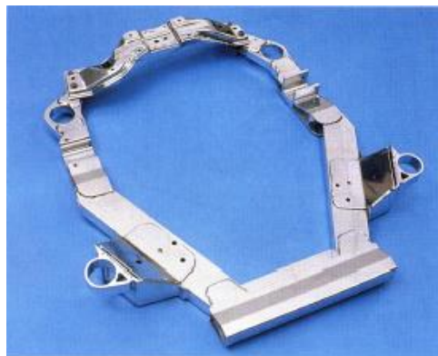
All-aluminium assembled engine cradle
