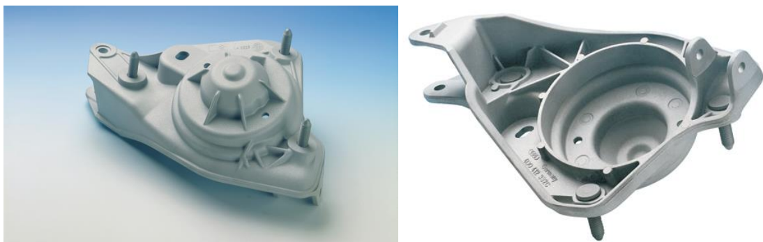
Early example of a suspension strut dome produced by vacuum high pressure die casting (alloy: GD-AlSi10Mg (A239))
