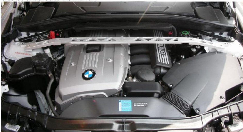
Cast aluminium strut bar (Photo: BMW)
