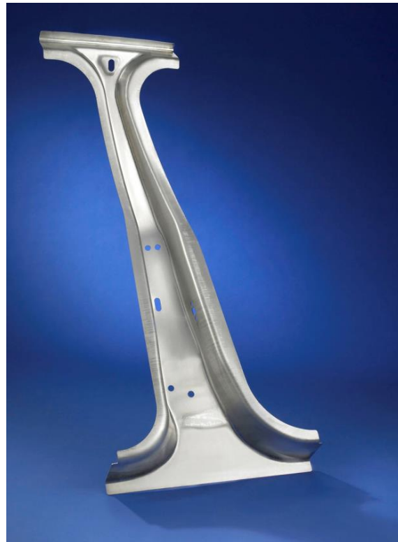
B pillar made using a 7xxx series ultra-high strength aluminium alloy (Photo: Aleris)
