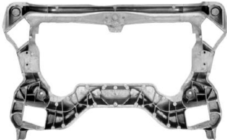
Cast aluminium engine cradle of the Mercedes-Benz C class (C204)
