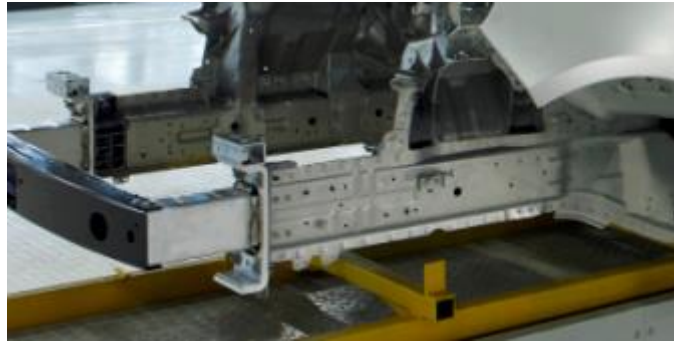
Application of the alloy Anticorodal®-300 in T61 temper in the Range Rover (L405) (Photo: Land Rover)
