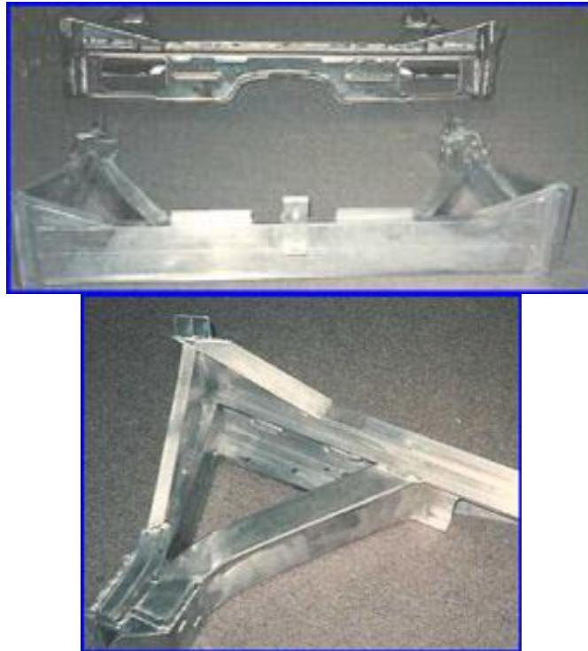
Comparison between the old, steel sheet-based frame and the aluminium extrusion design (left) and detail of the aluminium rear frame (right)
