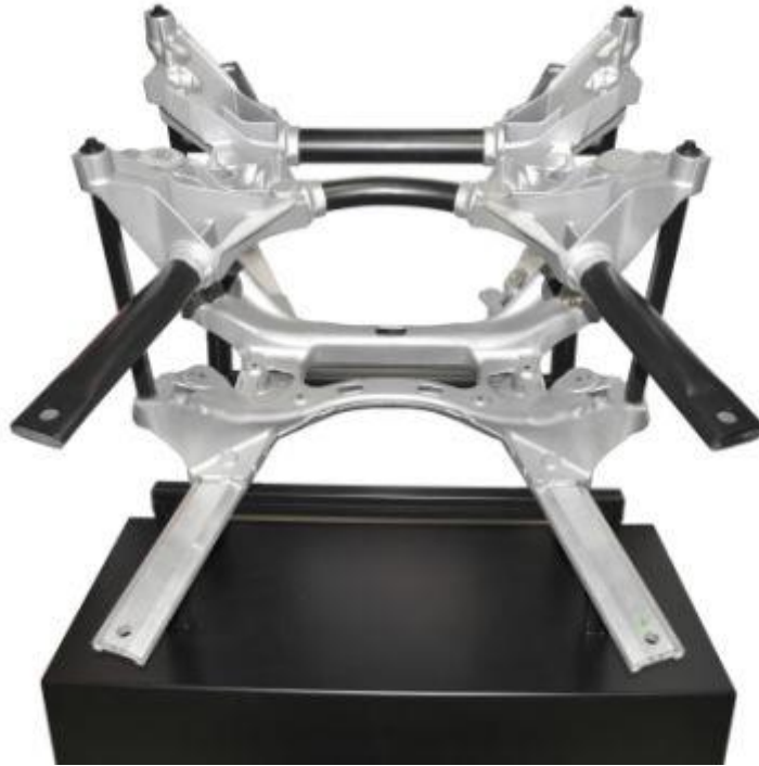
Bimetallic engine cradle with steel cross members and aluminium A356 cast over the tube ends
