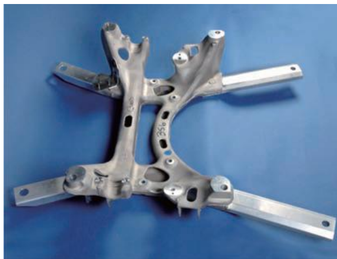
Aluminium engine cradle of the Cadillac CTS combining a large hollow casting with extrusions
