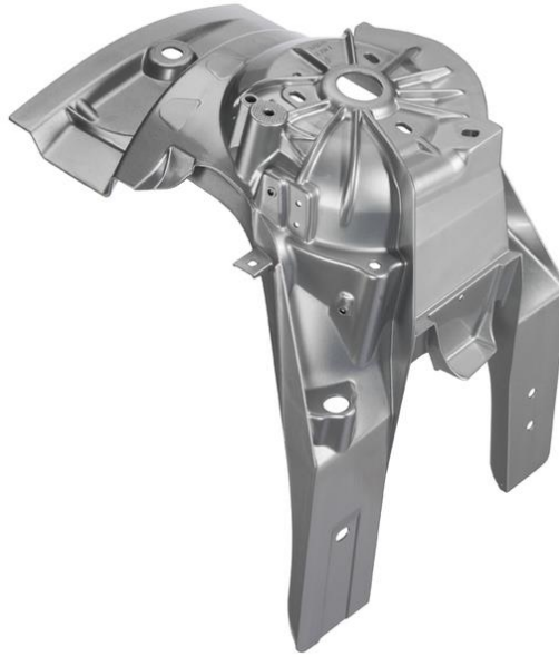
Aluminium suspension strut dome for the BMW 5 series models (Photo: GF Automotive)
