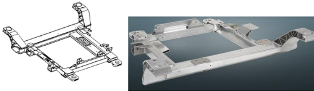
Extrusion-based aluminium engine cradle used for the Chevrolet Monte Carlo and Impala models
