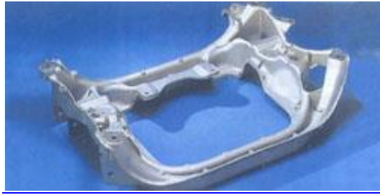
Cast engine cradle of the Mercedes-Benz S class (W220)
