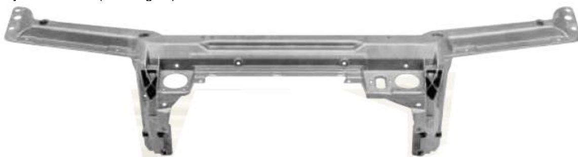
Front end carrier of the BMW 3 series convertible
