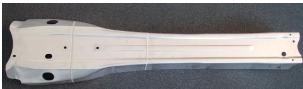
Tunnel of the Mercedes-Benz SL (R231) made using a tailor-welded blank (Photo: Novelis)
