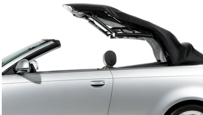
Retractable textile roof of the Audi A3
