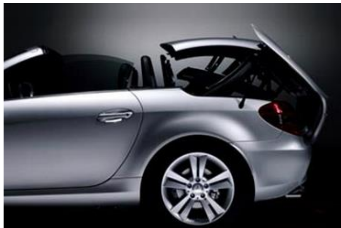
Three piece vario-roof of the Mercedes-Benz SL model (Photo: Daimler)
