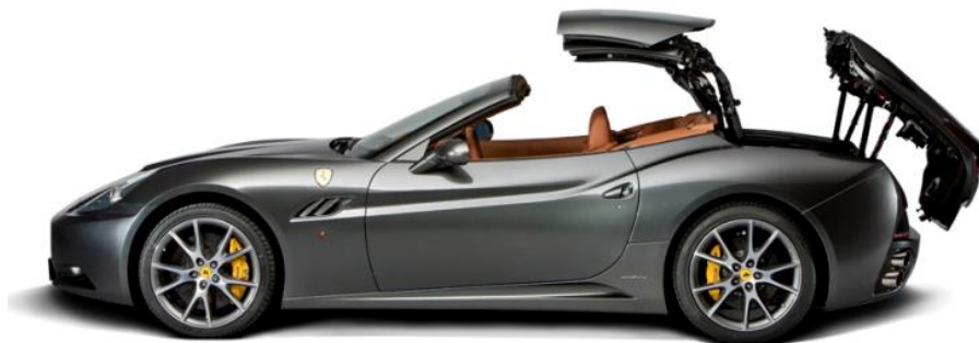
Retractable aluminium two-piece hardtop of the Ferrari California
