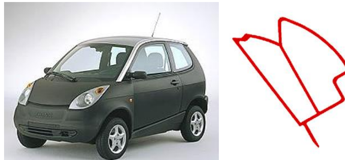
Ford THINK with an extruded aluminium cant rail
