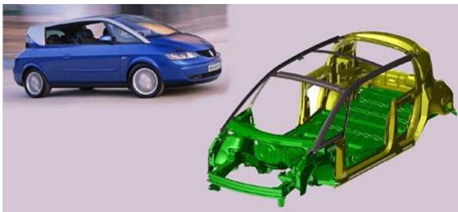
Body-in-white of the Renault Avantime (Source: Matra Automobile)
