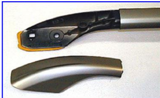
Roof rail support for mounting from the outside the vehicle with a removable cover
