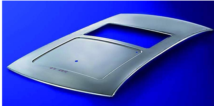
Aluminium roof of the Maybach luxury car (Photo: Maybach)
