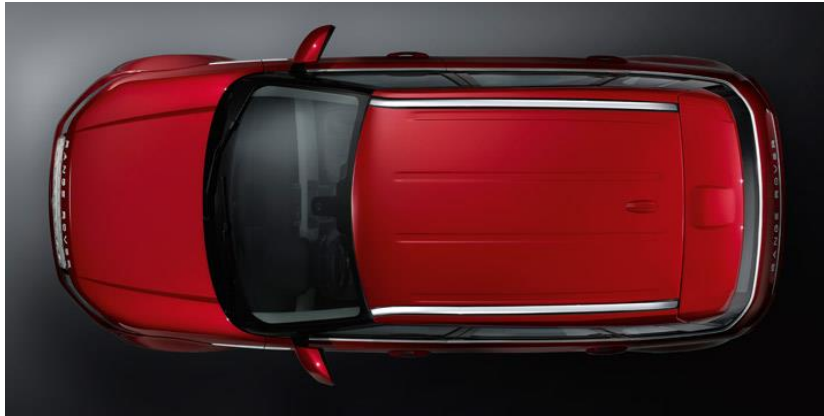
Range Rover Evoque with an aluminium roof (alloy: Anticorodal®-600 PX) (Photo: Land Rover)
