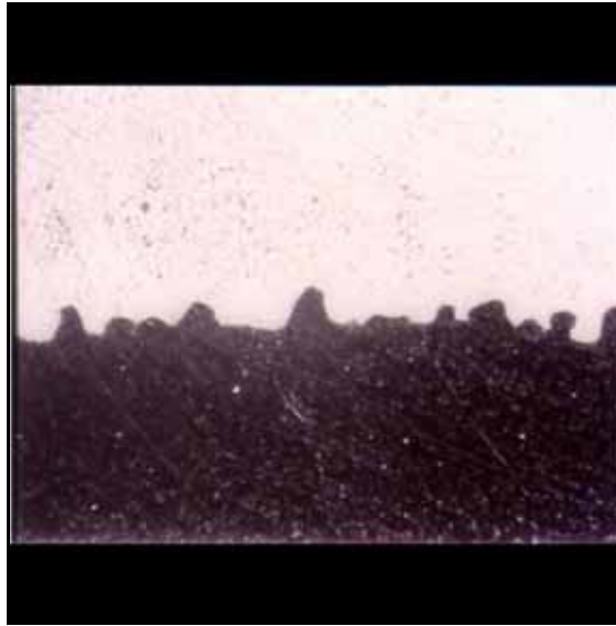
Micrograph demonstrating mechanical bonding between the cast aluminium alloy and the grey iron liner with a rough surface
