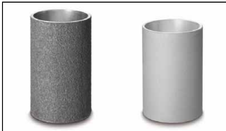
Grey cast iron liners with rough outer surfaces using either directly the as-cast surface (left) or a subsequent surface treatment (aluminium spraying) (right) ensure improved mechanical bonding
