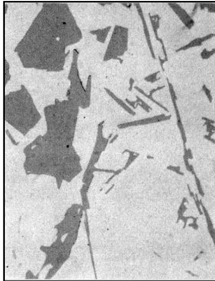
Micrograph showing as-cast microstructure of hypereutectic AlSi17Cu4Mg alloy
