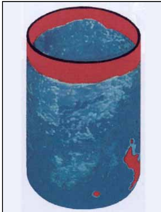
Ultrasound scan showing areas of good (blue) and bad (red) metallic contact
