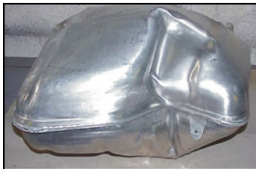
Pressure test with modified tank of a series production car (burst pressure 2.5 bar)
