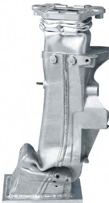
Deformed assembly of Laser - MIG welded high quality pressure die castings made from an AlSi casting alloy optimized for crash performance
