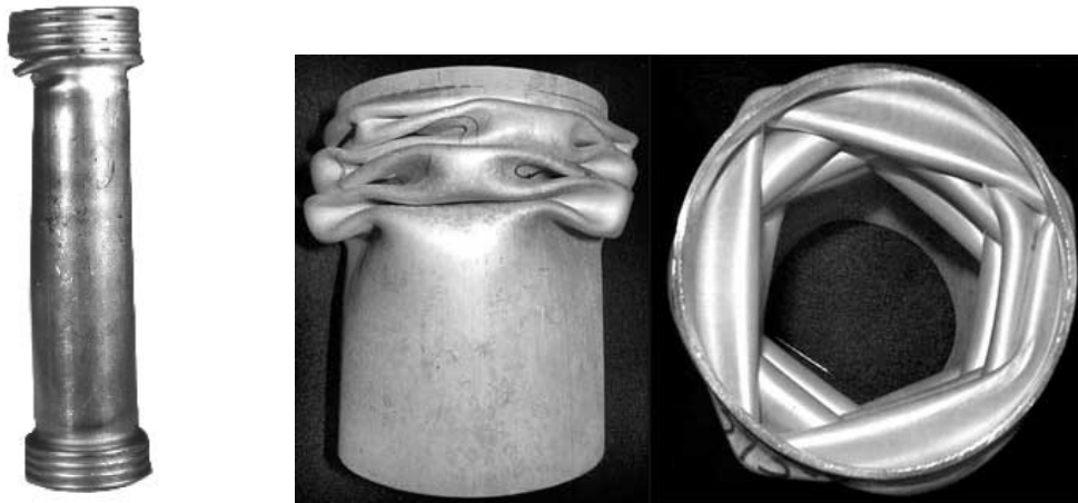
Axisymmetric (left) and diamond (right) folding pattern for circular crash boxes
