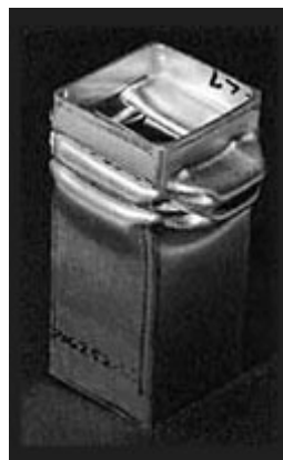
Quasi-static axial crush test results for a fan cooled 6063-T6 extrusion
