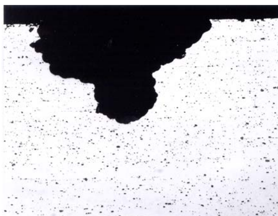
Local pitting corrosion on an uncoated aluminium sheet
