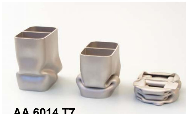
Deformation of an optimized extrusion alloy under axial crash loads
