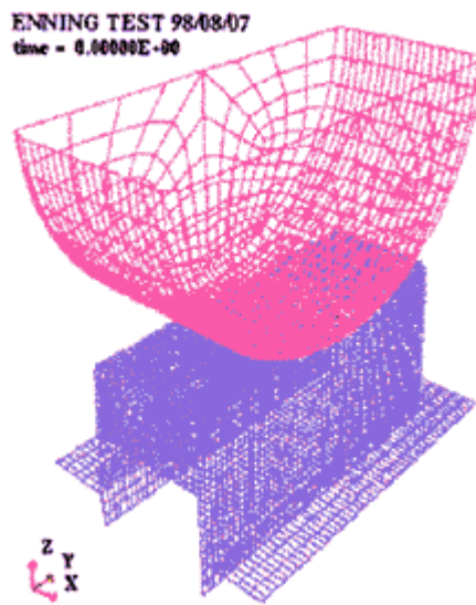
Configuration of crush test of CZ29-T6 hat-shaped casting
