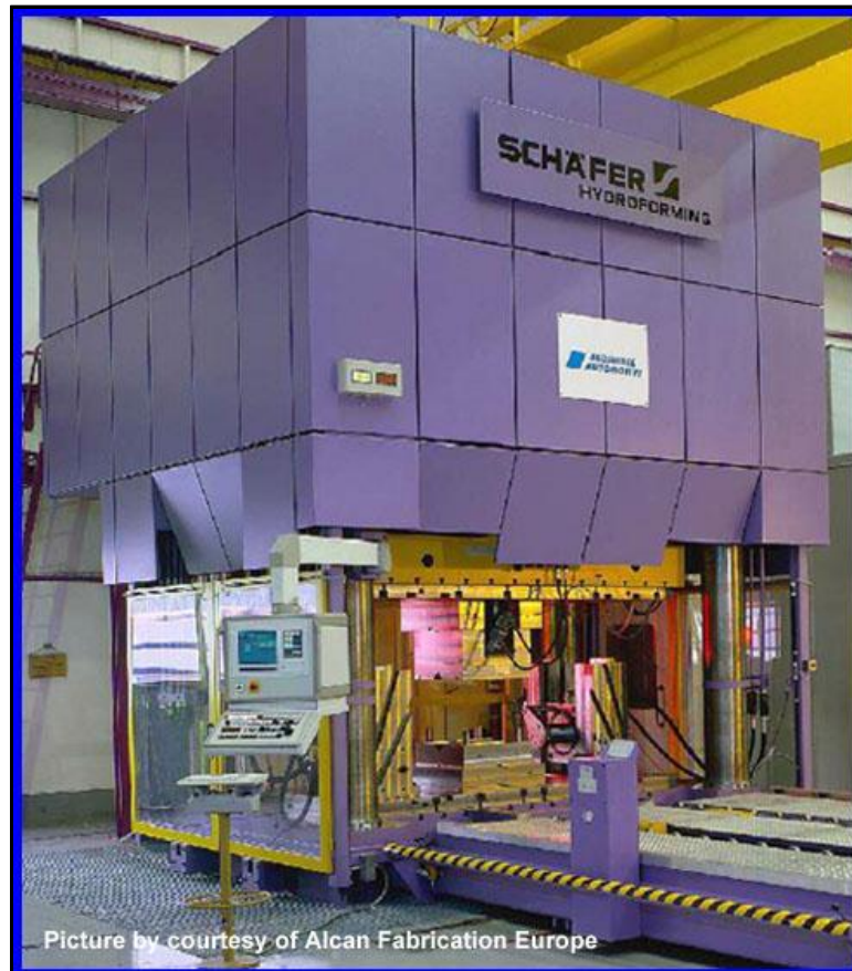
Example of a standard four column press (25.000 kN clamping force)
