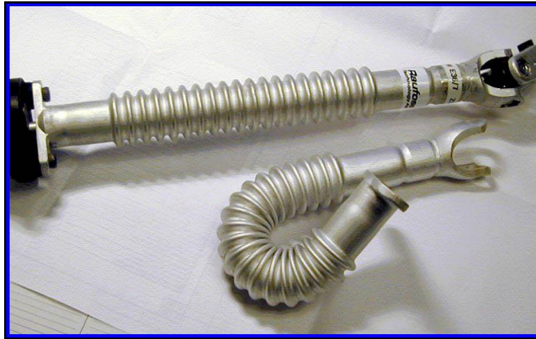
Steering shaft with convolutions
