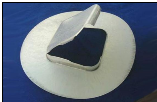
Square pan pressing of an uncoated blank using ~1.5g/m 2 of wax lubricant
