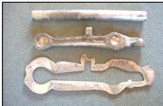
Forging stock (upper), forging (middle), sheared-off flash (lower)
