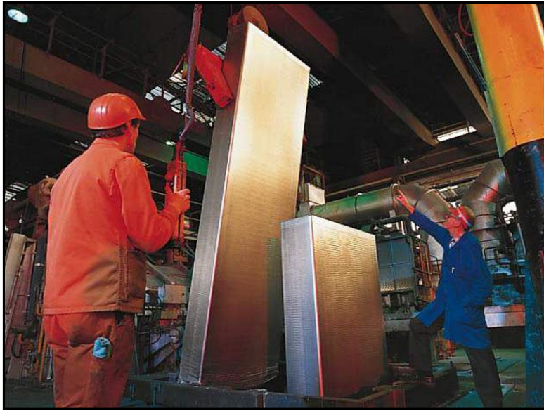
Rolling ingots are retracted from casting pit
