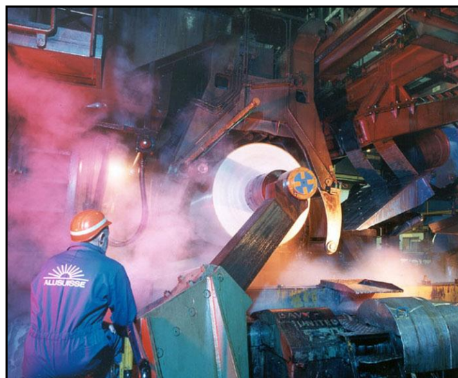
Coiling of the hot rolled strip
