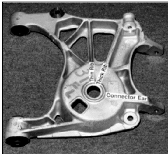
Lower Suspension Control Arm with Regions of Varying Thickness Marked for Comparison
